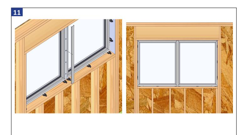
Snap the mull cover plate over base plate to finish off interior mull.
