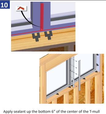
Apply sealant up the bottom 6" of the center of the T-mul filling the entire area as shown above. Insert the base plate with weather-strip flat against the window units and install with supplied bolts.
